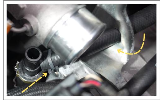
Route the drain hose under the AC hardline and through the bracket as shown.
