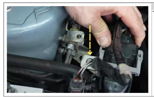
Step 32 Tighten harness bracket down.
