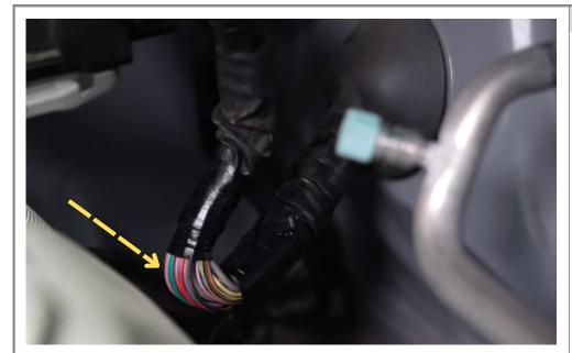
Use a razor blade to carefully trim electrical tape to release the branch of the harness.
