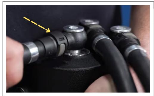
Attach the 26" drain hose to the AOS.
